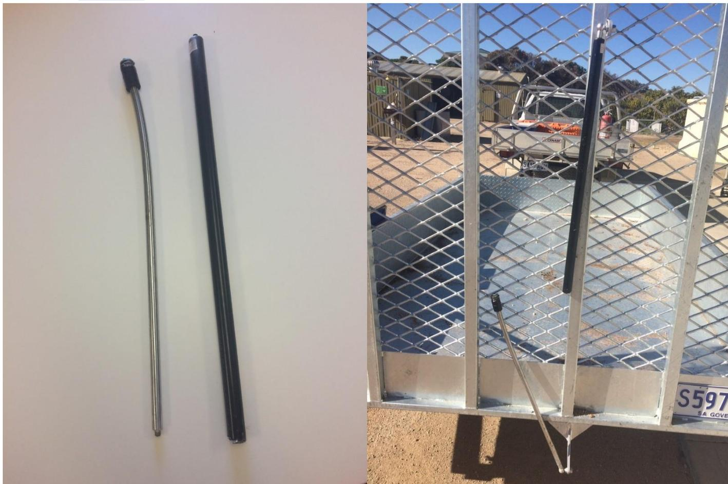
*Photo 2- the bent and broken gas strut (left) that failed while the tailgate ramp was being lowered (right).*
